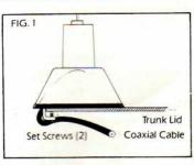
3. Route the coaxial cable from the trunk area to the radio. Install the PL-259 connector (supplied with TL kits). Connect antenna cable to radi
